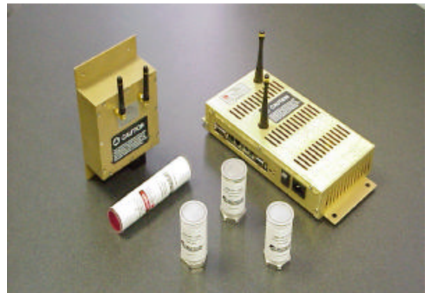
Figure 4 , Modern wireless CBM system including accelerometer, laser tachometer, and temperature sensors
